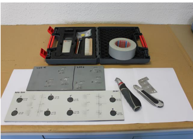
Adhesion by the cross-cut test
